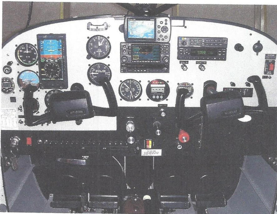
The completed IFR panel with products from Garmin, J.P. Instruments and Aspen Avionics.
